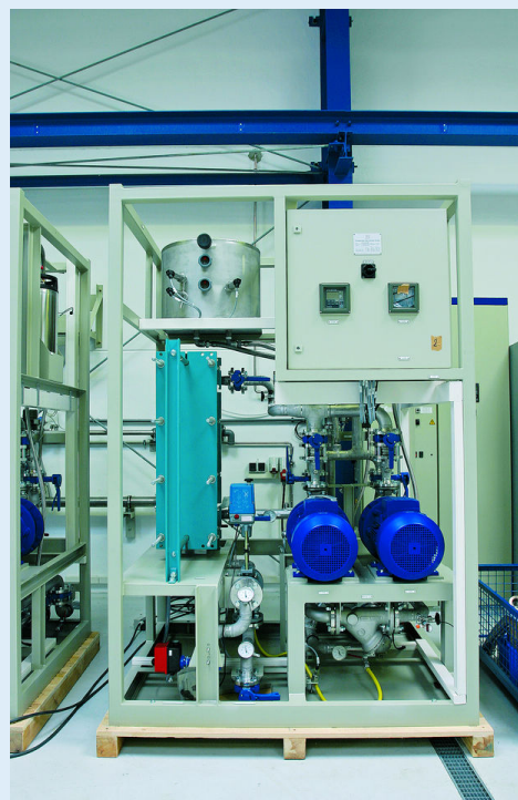
Cooling module built using construction kit system
