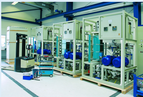
Cooling module manufacture for all rectifier and converter types at Anlagenbau Neundörfer GmbH
