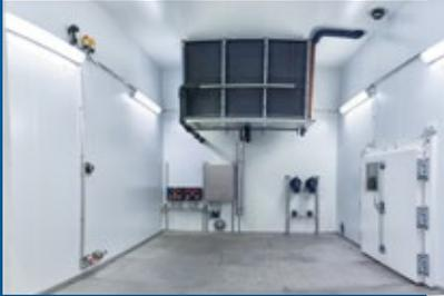
▲ Room temperatures of between -40 °C and +50 °C can be set in the test chambers at relative humidity levels of between 20 % and 95 %.
