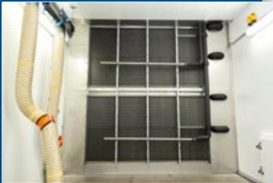
▲ 198 kW of refrigerating capacity and an air volume flow of 90,000 m<sup>3</sup>/h are installed in the large ATP test chamber. The fans have been optimised for use at between -40 °C and +50 °C.
