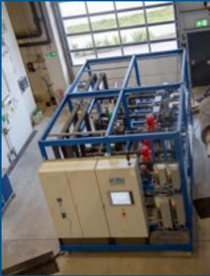
▲ TÜV SÜD's powerful CO<sub>2</sub> test rig in Olching delivers clear performance data, e.g. for condensing units and refrigerated display units.
