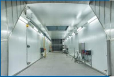
▲ ATP climatic chamber for testing refrigerated vehicles
