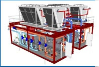
▲ The maximum tolerance at the flange connections in the prefabricated construction was just 5 mm owing to the confined space conditions.
