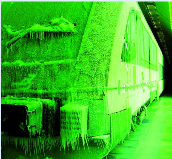
View of train in the Rail Tec Arsenal windtunnel in Vienna
